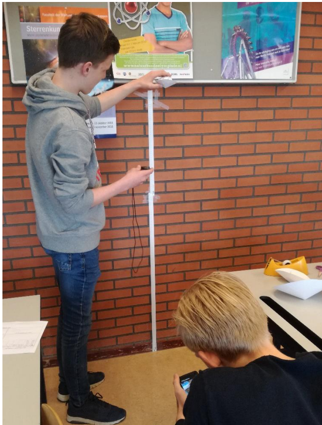
Figure 6. Students drop paper cones with different frontal areas and measure the falling time using both a stopwatch and their mobile phone camera.
