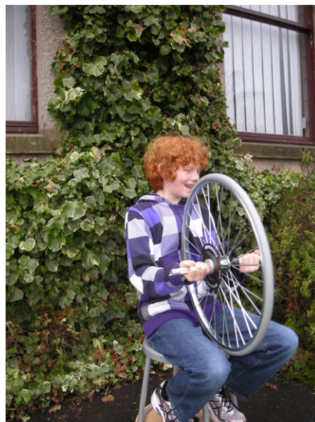
Figure 24. Using a commercially available gyroscope wheel from Pasco and rotating stool to demonstrate conservation of angular momentum.
